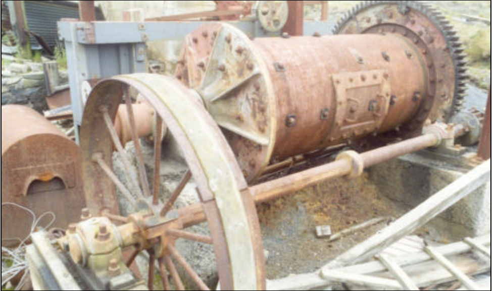
Ball Mill & lay shaft at Esgair Mwyn, June 2000 As previously used at Graig Wen gold mine (See last N/L, Item 44)
