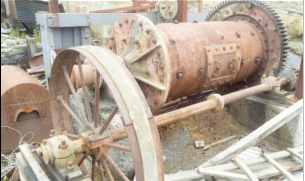
*Ball Mill & lay shaft at Esgair Mwyn, June 2000
